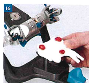
At the dental lab, the transfer table is placed in the articulator or the special mounting articulator used as a plastering device
