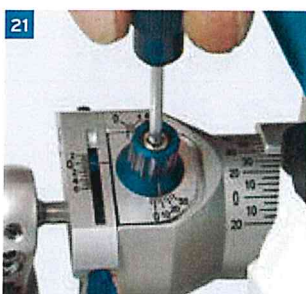
Open the side shift setting screw to open the ISS. Set the anterior guidance pin out of contact
