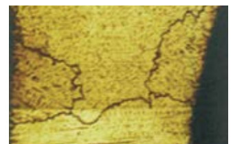
Coarse-grained structure of a conventional CoCrMo bonding alloy (magnification 100:1)
