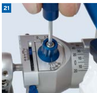
21 Open the side shift setting screw to open the ISS. Set the anterior guidance pin out of contact
