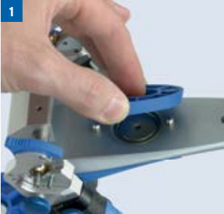
1 Remove model plates, magnets and magnet holders from the upper and lower parts of the Artex articulator
