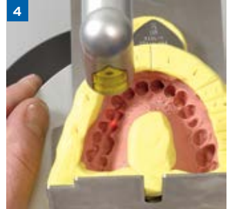
4 Position drilling hole with the aid of the laser beam and initiate drilling procedure
