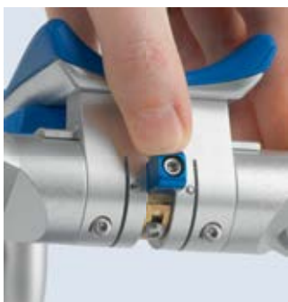
The reproducible centric guarantees a reliable start and end position of each excursion. Interferences less than 20 µm can be identified, checked and removed
