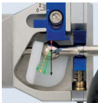
The reproducible centric guarantees a reliable start and end position of each excursion. Interferences less than 20 µm can be identified, checked and removed
