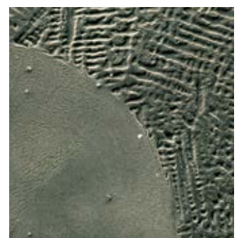
Laser weld without any cracks in a carbon-free CoCrMo alloy
