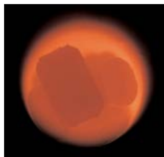
Begin of the melting; the casting cubes melt into each other
