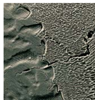
Cracks caused by carbide precipitation in a CoCrMo alloy containing carbon
